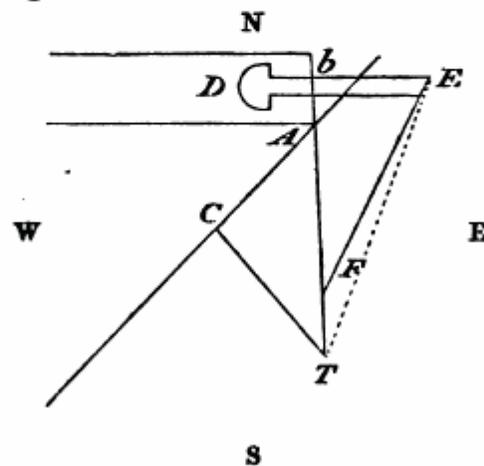
The true style  $CT$ ,  $50\frac{1}{4}$  lines in height, must have been, at  $C$ ,  $48\frac{1}{5}$  lines from the angle  $A$  of the marble, in the eastern dial.
