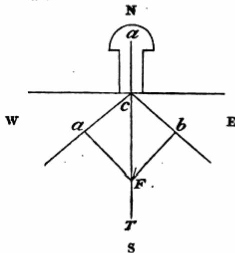
For the southern dials the arrangement was more simple ; the style *CT* was the continuation of the part *ac* fixed in the wall : it might have been strengthened by the addition of the quadrilateral figure *caFb*, filling up the space on each side of it ; the point *F* would give the time of noon at the solstice, and *T* would point out all the other hours by its shadow.
